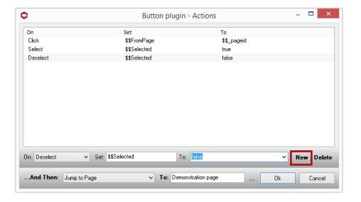
Once the parameters have been set Acquire will continuously monitor the state of buttons and perform an action on detecting a change in button state.
